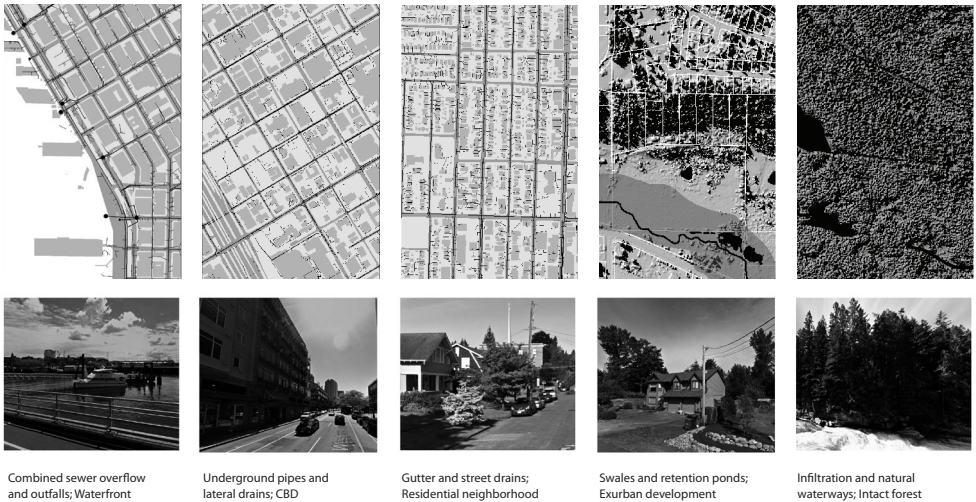
FIGURE 5.2 Urban hydrology has implications for urban infrastructure across a gradient of urbanization. Maps (left to right): LiDAR Top Surface DEM 2003: King County, Washington (2003); infrastructure, sewer, and drainage: City of Seattle 2012; property/survey: building outlines (City of Seattle 2012), street/transportation: City of Seattle 2012. All photographs: Google Maps 2015.
